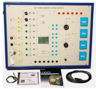
The PLC trainer provides to the student the ability to study the Programmable Logic Device applications in the Industrial and Modern Home automations .
