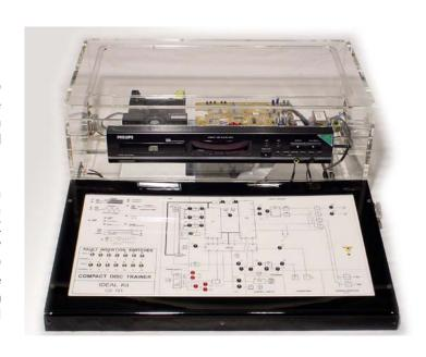
At the front side of the unit there is a panel (dimensions in cm 61W X 34D) with the circuit (block) diagram of the CD. Throughout the most suitable parts of the CD Player's circuit are the test points of the CD system for connecting various instruments (oscilloscopes, etc) for the acquisition of the necessary waveforms.
