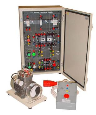
With the one phase motor trainer one can study the automated change of the direction of rotation of a one phase motor .
